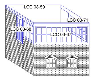
Next step in assembly is gluing the laminates to the signal box body. Start with LCC 03-68 and LCC 03-71. Follow with the two remaining elements. Ensure that the parts marked blue are glued in flush with the outside of the signal box.
