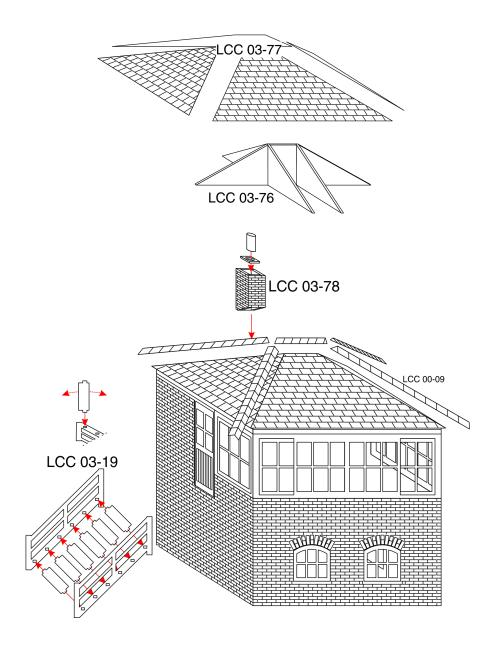
Remove roof support parts LCC 03-76 from their spruce and glue together by slotting together as shown on picture above. Leave them until glue dries prior making sure they are all at right angles to each other. Take out LCC 03-77 roof panels from their spruce and start gluing them to the supports. Assemble on a flat surface ensuring the roof is square on edges and flat on the bottom.
